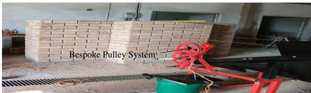
Figure. 3: Non-straight wall testing: (a) Schematic figure and (b) Test setup displaying system for lateral load
