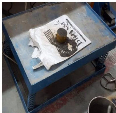
Figure 1: Determination of packing density using vibrating table
