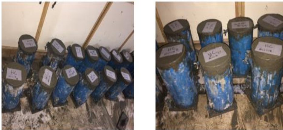
Figure 4: Casting of Test Specimens
