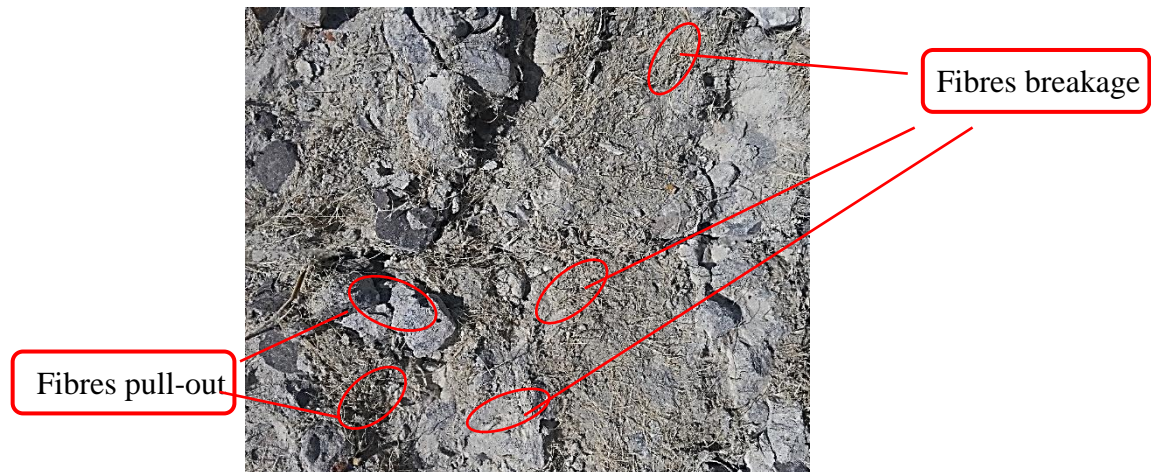
Figure 4: Fibres breakage and pull-out behavior
