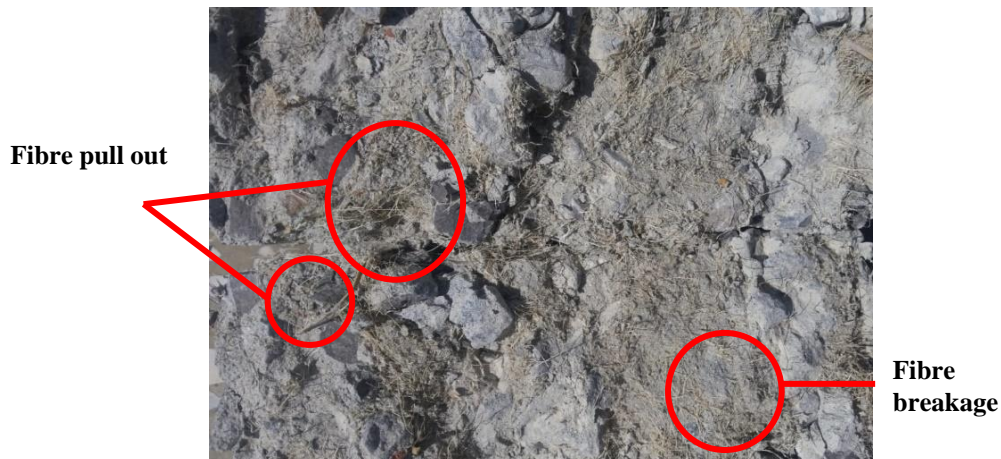
Figure 4: Fibre behavior in broken test specimen
