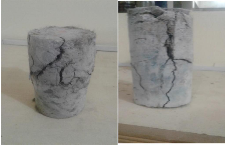
Figure 2: Failure pattern of concrete cylinders
