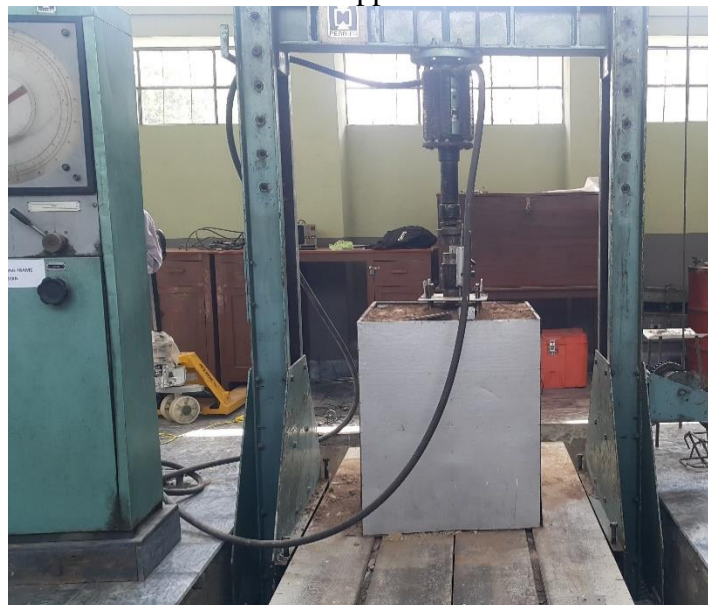
Figure 3: Loading strain frame
