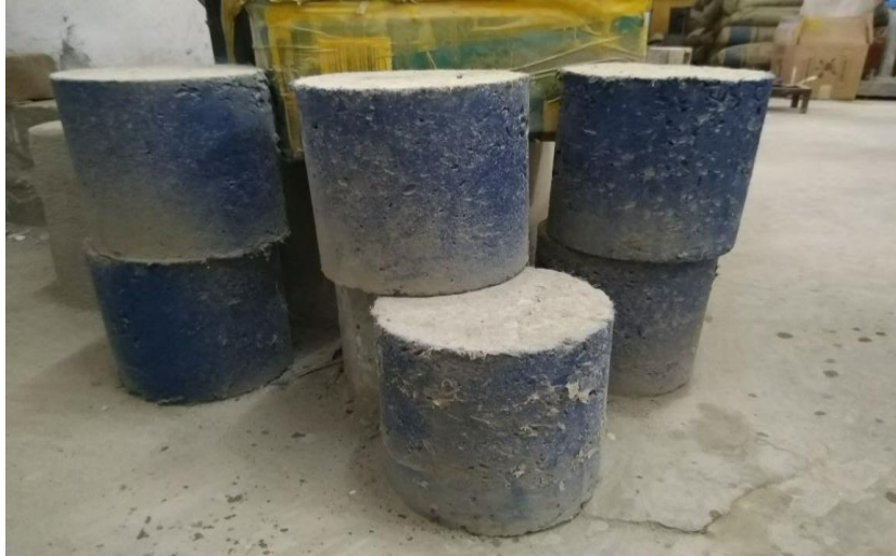
Figure 5: Application of Blue Emulsion pain to prevent penetration of water from sides
