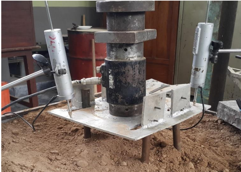
Figure 2: Instrumentation of Pile Group Model
