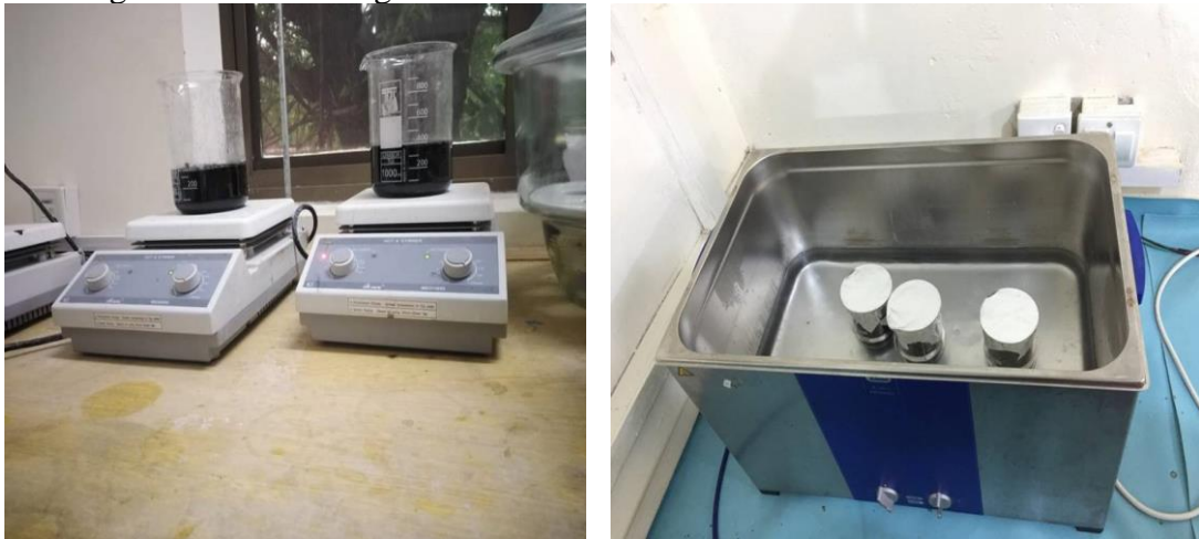
Figure 1: (a) Stirrer mechanism; (b) Bath sonicator
